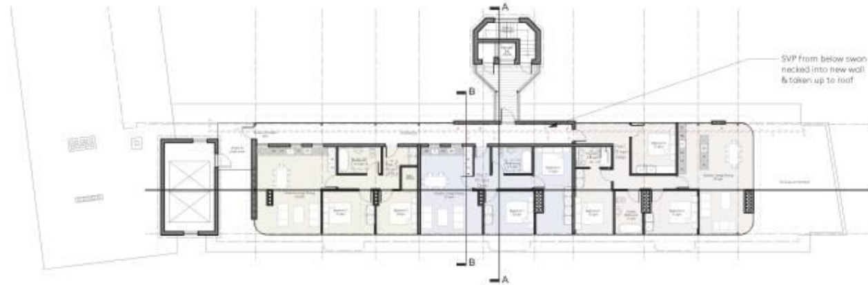
2 Proposed 6th Floor Plan Scale: 1:200
